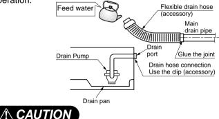
The supplied flexible drain hose should not be curved, neither screwed. The curved or screwed hose may cause a leakage of water.
